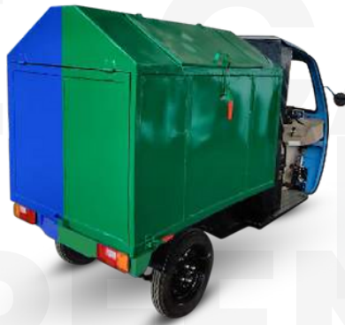
E Cart with Garbage Box with Dry/Wet Compartment % Hydraulic Tipping Mechanism
